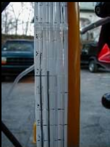
A cheap set of carb sticks. Marked in centimeters of mercury, these are very sensitive. Most manufacturers request balance less than 2 cm Hg. Up to four cylinders can be viewed side-by-side.
